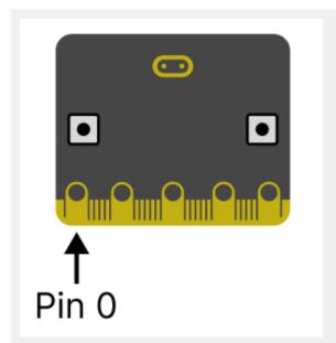
Just like buttons A and B, your micro:bit also has several **pins** which you can use to interact with your pet. For this challenge, we'll be using pin 0, which is at the bottom left of your micro:bit.
