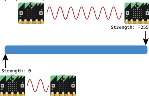
If we check the signal strength of messages that we get, we can compare it to the strength of a micro:bit that is kind of close to you. You can test this yourself and tweak the value, but we find that -35dBm is a good number!
